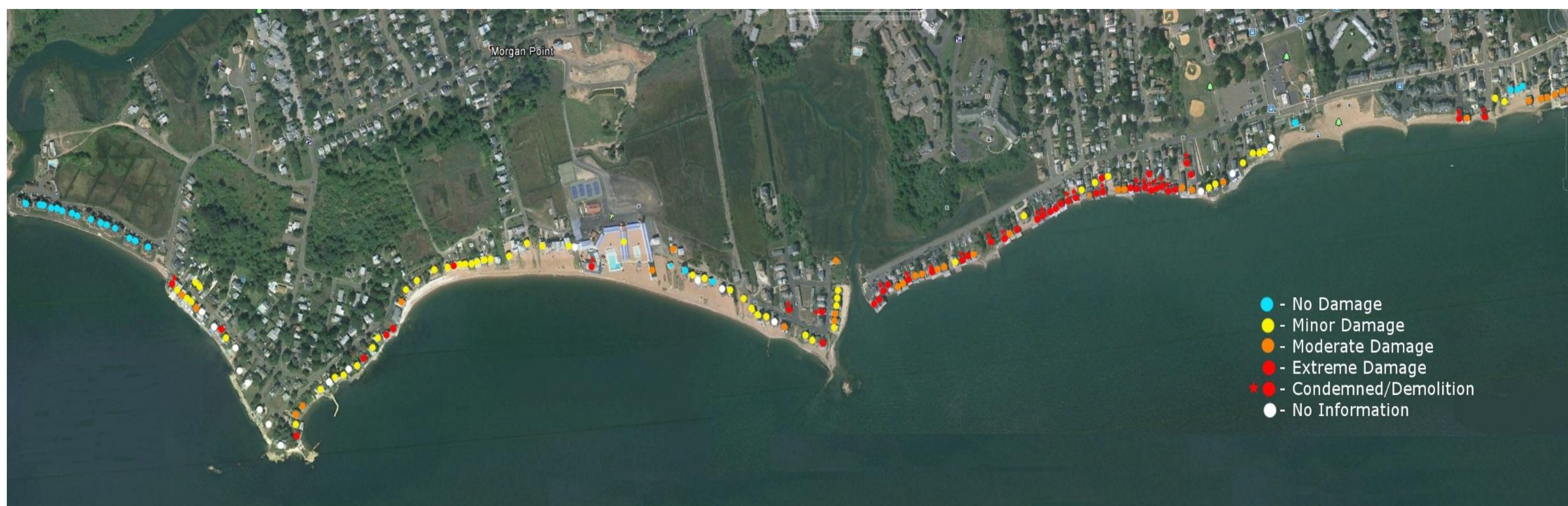
This map illustrates the damages to homes along the East Haven shoreline during Sandy based on interviews conducted by Stephanie Cherry in conjunction with data from town records.
