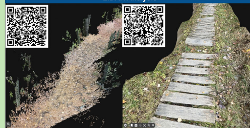
Figure 11: LiDAR gives researcher a detailed texture of each trail. Although the wood board made the trails partially inaccessible for wheelchairs, etc., it minimized the trail's impact on the environment and protected the underneath vegetation.
