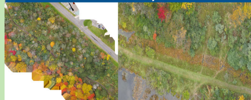
Figure 10: Utilizing corridor flight modes, researchers gain a thorough overview of the condition of Marsh trails. Most hikers enter the preserve through the Marsh trail and depart at the intersection to view the bridge. The two images demonstrate that trails experiencing higher foot traffic tend to exhibit more pronounced bareness and erosion compared to less frequented areas.
