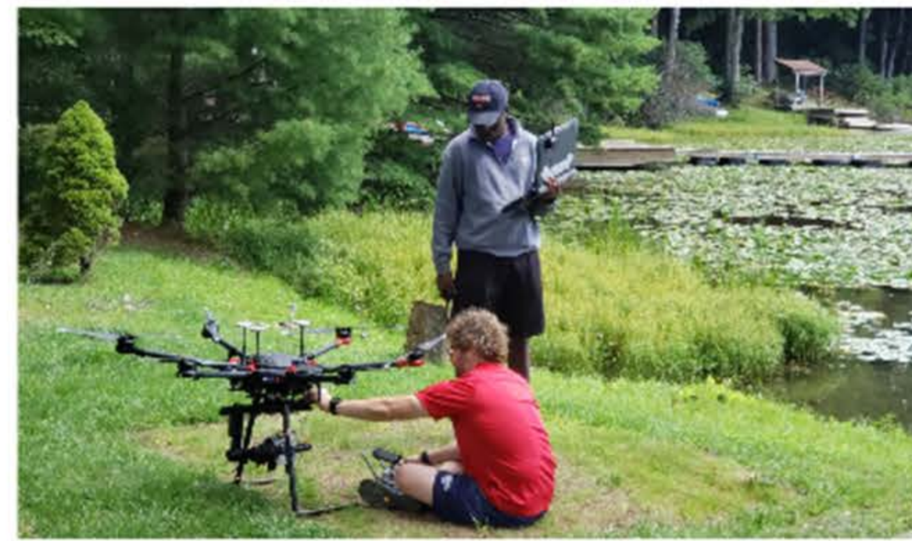
Figure 2. Setting up UAV with Toughbook computer ground control station.
