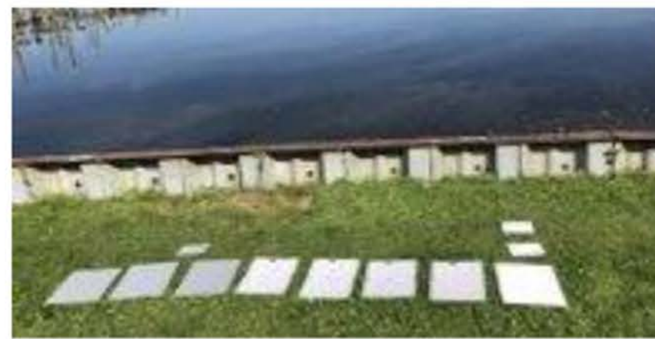
Figure 3. Field set up of calibration cards at launch site.
