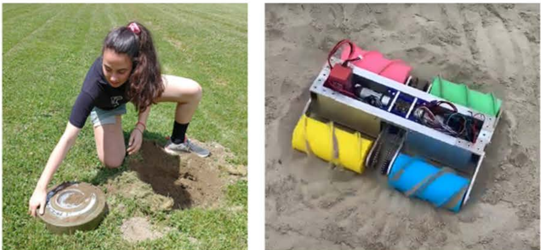
Figure 2: TM-62 field test site at Binghamton; Figure 3: "Fruit Loop" the robot designed to carry an MFAM under vegetation
