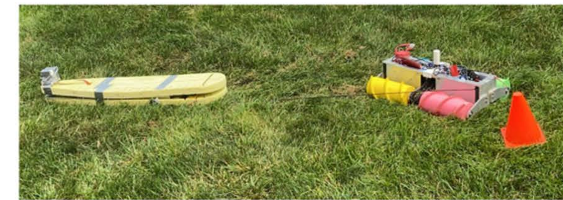
Figure 4: The "snake bot" system: robot designed by Villanova and Binghamton University student carries behind it an MFAM magnetic sensor over a field of TM-62 mine shells. If this method works to produce images that detect mines, it can be used to prevent land razing by traveling under vegetation to detect mines.
