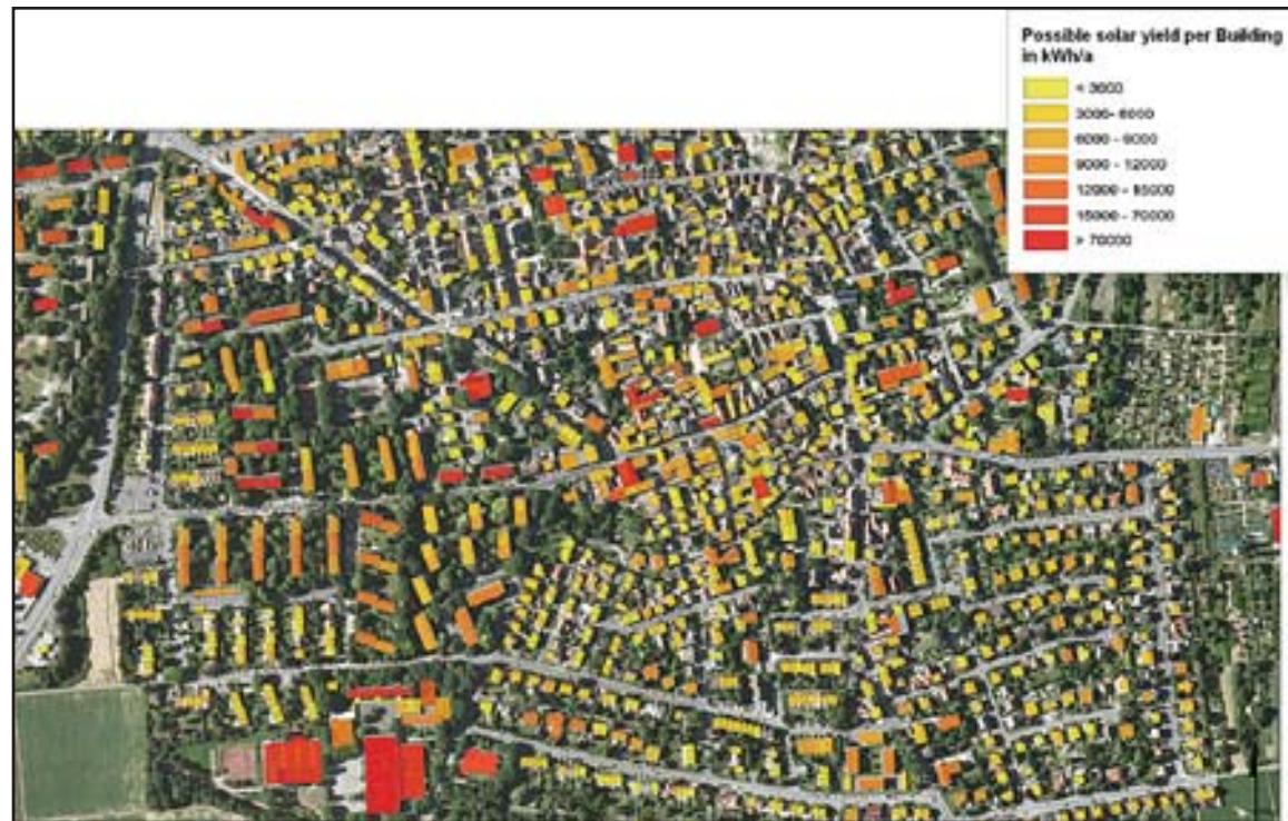
SUN-AREA researchers used ArcGIS Desktop applications to calculate the possible solar yield per building for the city of Osnabrück.
