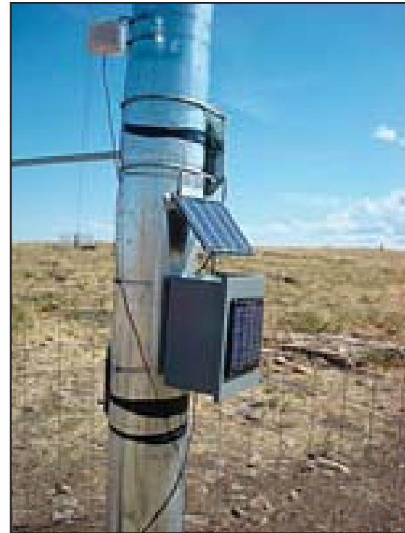
Wind data from sensors on this rural anemometer is sent to remote computers for analysis.
