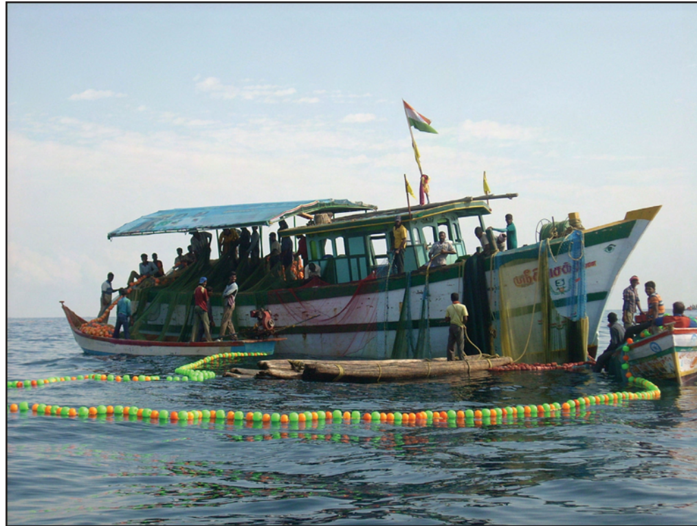
A large mechanized boat comprising up to 80 fishermen. The ring seine net often extends for kilometers, therefore resulting in considerably large catches of sardines or mackerel.
